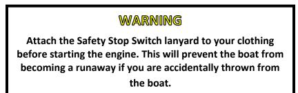
The Safety Stop Switch can only be effective when it is in good working condition. Observe the following:
